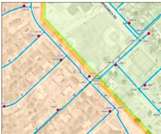
On this sample water system map, red dots represent hydrants and blue lines identify the the pipes.
